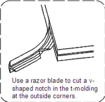
Use a razor blade to cut a v-shaped notch in the t-molding at the outside corners.
