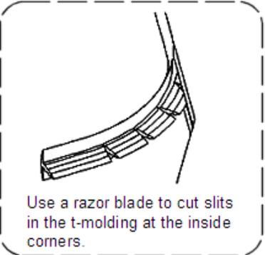
Use a razor blade to cut slits in the t-molding at the inside corners.
